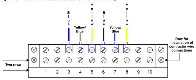
The recommended gauge for Status/Control Connection wires is 16 AWG – 600 VDC (approximate metric equivalent: 1.3 mm² wire section). All wiring must comply with all applicable local, regional, national regulations.
